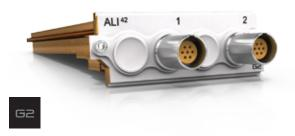
The ALI42 G2 Module is a 2 channel high speed Module with sample rates up to 819.2 kSa/s. Both channels operate independently of each other, each with its own mode, gain, coupling, etc. and with all settings done in software. The ALI42 G2 has two 7-pin Lemo connectors and can be used for both high bandwidth analog input as well as full bridge measurement applications.
