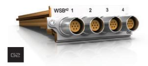
The WSB42 G2 Module is used with AC and DC bridge measurements including strain gauges configured as full, half or quarter bridges and inductive displacement transducers (LVDT). The Module offers numerous software selectable features such as constant voltage excitation (AC or DC), bridge sensing, bridge completion resistors and shunt calibration. The bridge can be balanced on command or a previous balance value can be recalled.
