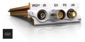
In addition to the same internal GPS functionality as described in the GPS42 G2, the IRG42 G2 Module provides an additional functional unit of being able to interface to IRIG. Here IRIG-A and IRIG-B data (both analog and digital formats) are digitized by a high speed ADC and decoded. The external IRIG data is time-stamped to synchronize its data with other Modules in the same system.
