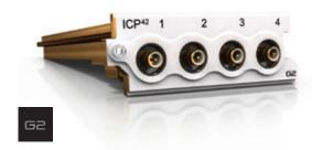
The ICP42 G2 Module can be used with ICP® based accelerometers, force and pressure sensors as well as to measure analog voltages. All 4 channels operate independently of each other, each with their own setting of mode, gain and coupling.
