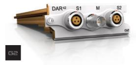
The DAR42 G2 Module provides interfaces to receive two stereo AES3 digital audio streams. For synchronization between the DAR42 G2 and external digital audio transmission equipment, the DAR42 transmits a synchronization signal which can be selected to be either an AES3 output signal (data at digital zero) or word clock signal.
