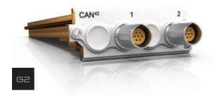
The CAN42 G2 Module provides interfaces to 2 independent Controller Area Networks or CAN. Messages received from CAN are time-stamped to synchronize their reception with analog and digital measurements from other Modules in the system. Fully implemented features include Listen-Only mode, Self-Reception of CAN messages and transmission of Remote Frames. The CAN42 G2 Module provides independent channel filtering.
